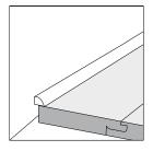
A suitable edge trim of your choice can be used to cover expansion gaps. These should be fixed to the skirting or wall and not to the flooring.
