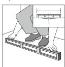
Amtico Click can be installed over stone, vinyl, linoleum or laminate flooring, but carpeting must be removed. Concrete slabs and stone floors may be uneven and have high levels of moisture, which will require correction. If the subfloor is rough or uneven, this could create an unsightly appearance to the finished floor, and should be corrected using a suitable leveling compound on a concrete base, or by overlaying with plywood on a wooden base.
