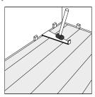
The use of a pullbar in conjunction with a rubber mallet is recommended for ensuring the tongues and grooves of the final two rows are well connected.
