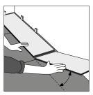
Attach the second plank by laying the end connection at an angle accurately on top of the first plank and drop into position ensuring that the long edges of both planks are aligned.
