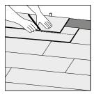
To lay the last row the distance between wall is measured and planks can be cut to size, again allowing for expansion gaps.
