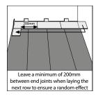
**TIP:** The offcut from the first row can be used as the first plank in the second row if the joints are well separated.
