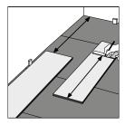
**TIP:** If the last plank is less than 200 mm in length, it is recommended that a small section be cut from the other end of the row, which can then be slid across the room to create space for a larger infill of plank. For stone tiles set these out in a Brick fashion.
