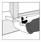
Skirting boards may be removed and door frames undercut if required, to allow for possible expansion of the finished floor ensuring there is an allowance for expansion under the door frames.
